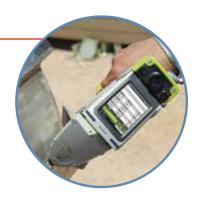
Analyze nearly every element of interest in virtually all types of metal alloys, from tramp elements to pure metals, and everything in between. With point-and-shoot simplicity, you can view the alloy grade and chemistry on the built-in, color, touch-screen display.
